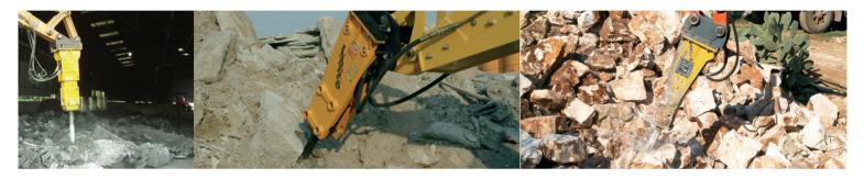
breaking in quarries, as well as for more specific tasks. In fact, midi range breakers are used for underwater work - using a special kit - as well as for digging narrow deep trenches and removing casting slag from blast furnaces.
